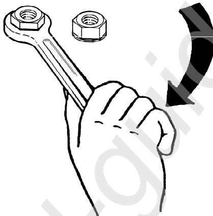
Fig. Checking bolted joint
